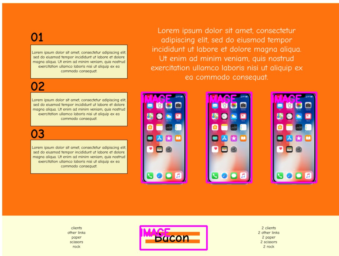
Figure 4.13: Results of Image Detection Using Template Matching Technique. The individual elements — the smartphone and the logo — are accurately positioned within the web design template. This precision is evidenced by the congruence of size and location in relation to the encompassing elements of the design.
