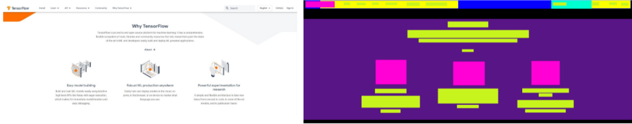
Figure 2.8: On the left, an image of the webpage design is displayed, representative of the first dataset, which includes the primary web elements. On the right, an illustration of the segmented dataset is shown, comprising labels for 'divs' and 'sections'. The use of this segmented dataset aims to enhance the accuracy of the detection algorithm.
