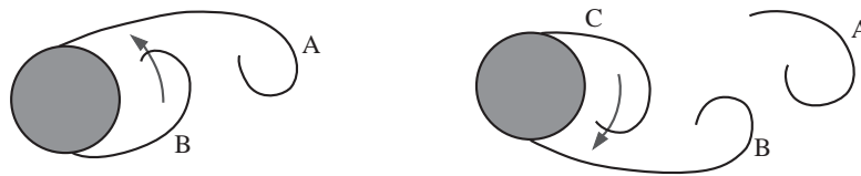
Figure 2.3: Vortex shedding mechanism. In the first scheme, the vortex A is larger and throws the vortex B across the wake. In the second scheme, the vortex B has grown enough to throw the vortex C across the wake. This mechanism is repeated in an alternate manner at each side of the cylinder to form the “vortex street”. Based on Sumer & Fredsøe (1997).
