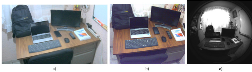
Fig. 2. Example images of the office scene: a) Webcam Perfect Choice, b) iDS, c) Intel RealSense T265. All cameras are located at the same reference point.
