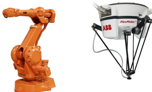
(a) Robot serial ABB IRB2400 (tomado de [ROBOTRADERS, 2017]). (b) Robot paralelo ABB IRB 360 (tomado de [Robotics, 2017a]).
