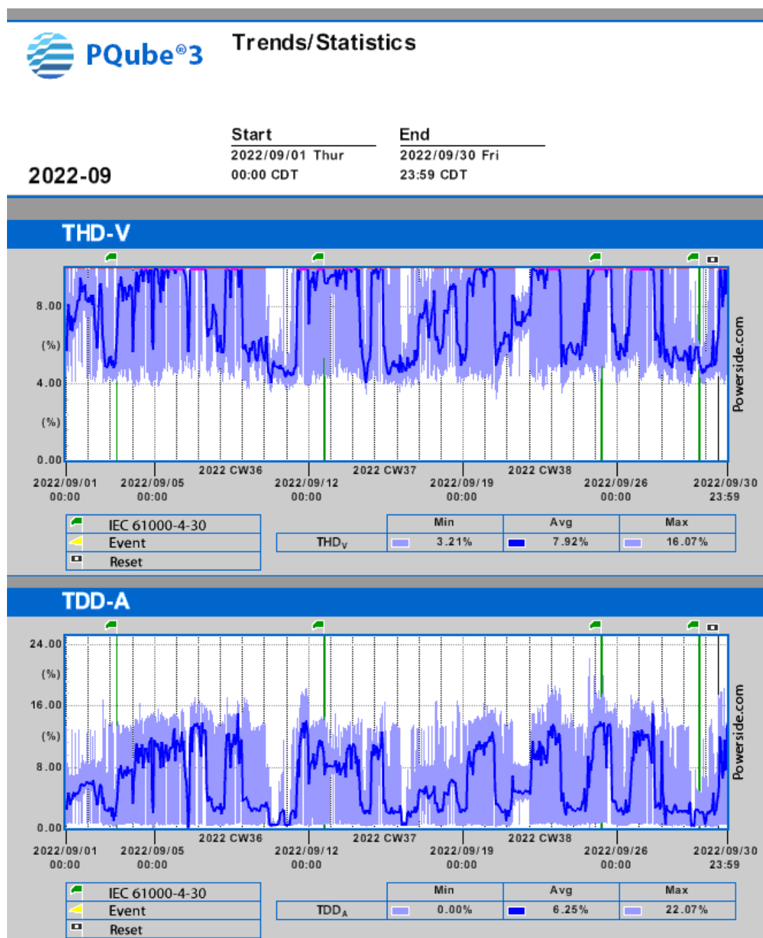
Figure 4.4: One month trending for drilling rig #2, with shunt harmonic filter tuned on the 5th harmonic.
