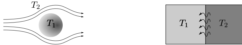
(a) Heat transferred due to convection (b) Heat transferred due to conduction
