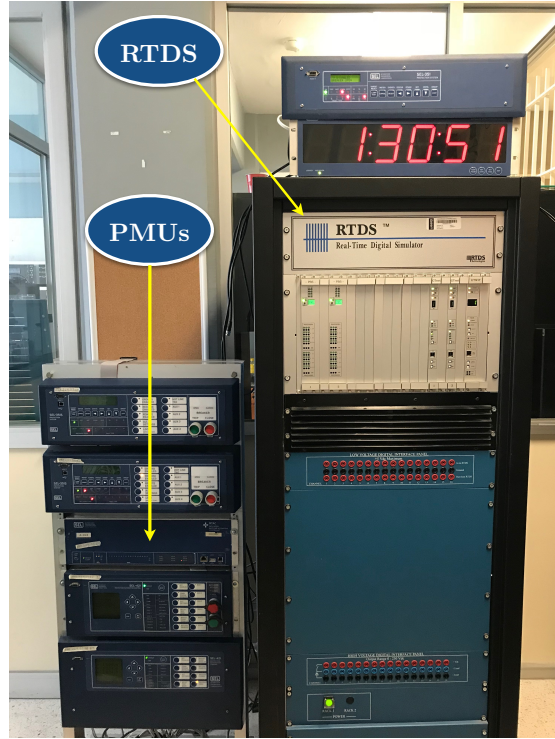
FIGURE 5.3: Hardware-in-the-loop implementation in RTDS.
