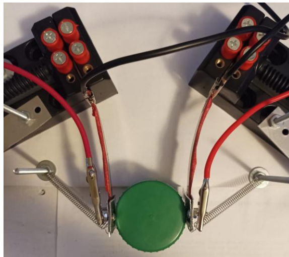
Figure 6-45.- Case study 1 gripper prototype in the austenite phase.
