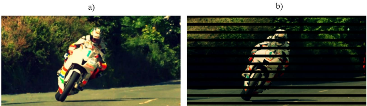
Figure 4.12. The idea behind the blinds method. a) Original frame, b) same frame after applying the blinds method
