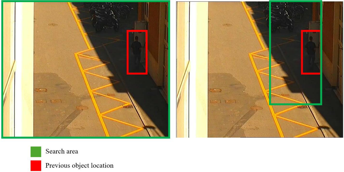
Figure 4.10. Change on the search area with the four predetermined percentages based on 3 times the object size radius (75% up, 50% down, 50% left, 99% right)
