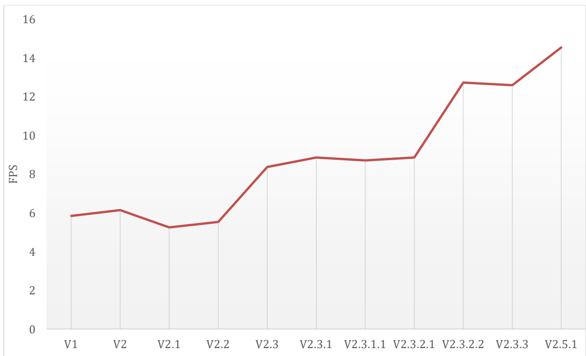
Figure 5.2. Speed graph of the single ZNCC parallel versions
