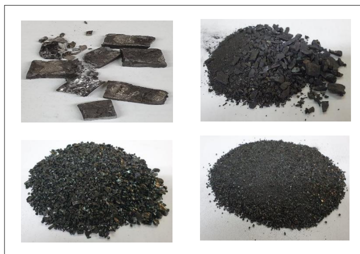
Figura 32. Prueba 17, metal (169.99 g), mata (73.40 g), escoria + 10 m (189.30 g) y escoria -10 m (154.78 g).
