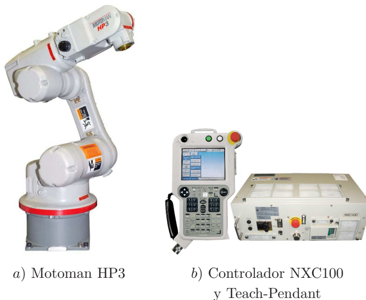
Figura 4.9: Robot serial MOTOMAN HP3 de YASKAWA Company.
